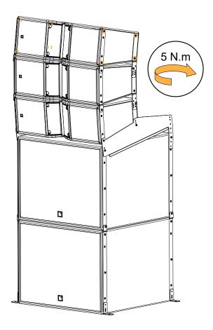
**14.** Check that all screws are secured and tightened.
